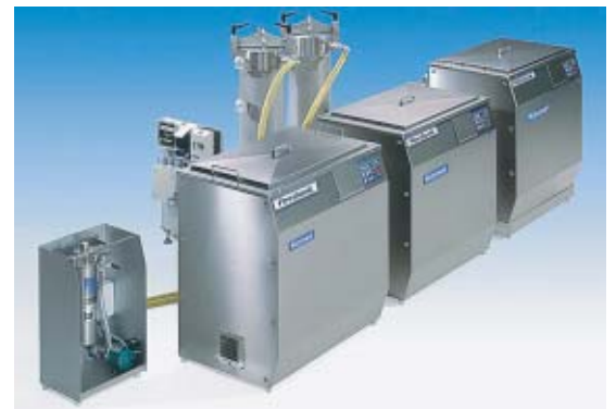
Si-80 wash stage with 10" filter and two stage cascade rinse with P2S size closed loop filtration, active carbon filter and deioniser.
