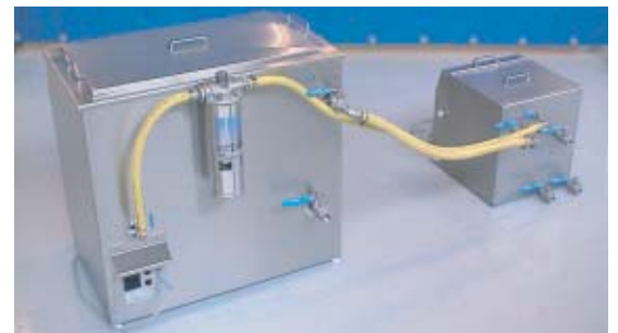
Storage tank with oil separation unit.
